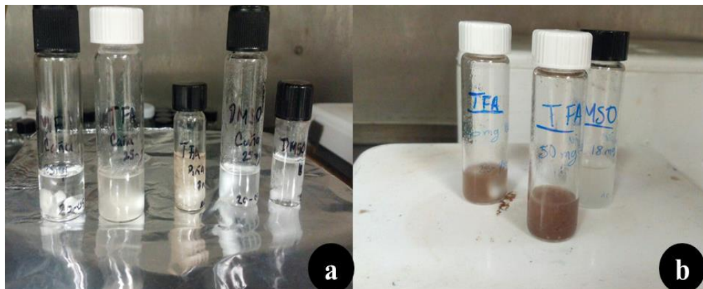
Fig. 4. Cellulose samples at 2.5%, 3.3% and 10%, respectively, using TFA as solvent, with respect to w/v.
